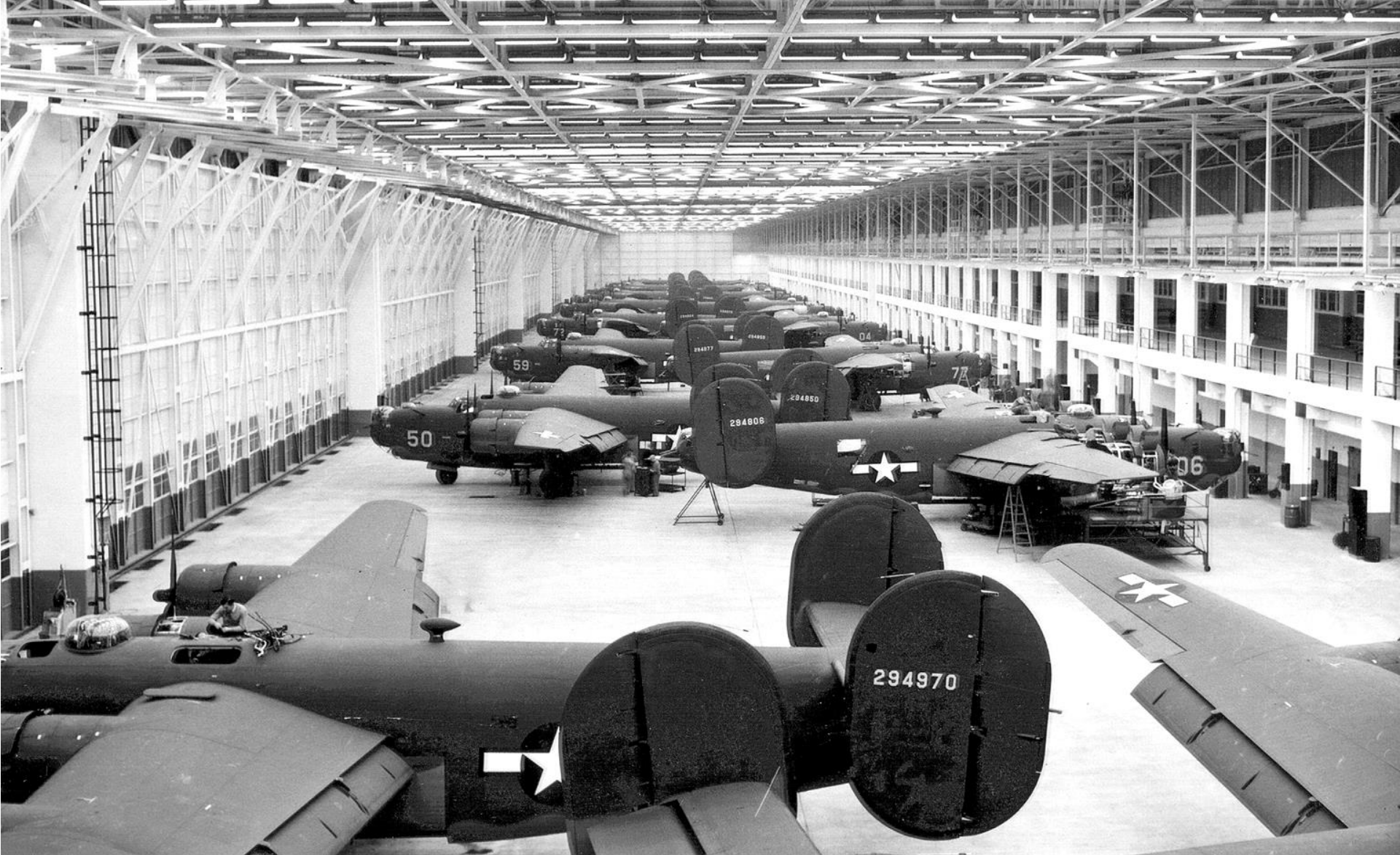
The "Arsenal of Democracy": Ford Willow Run Plant Producing a B-24 Liberator Bomber every 55 Minutes
